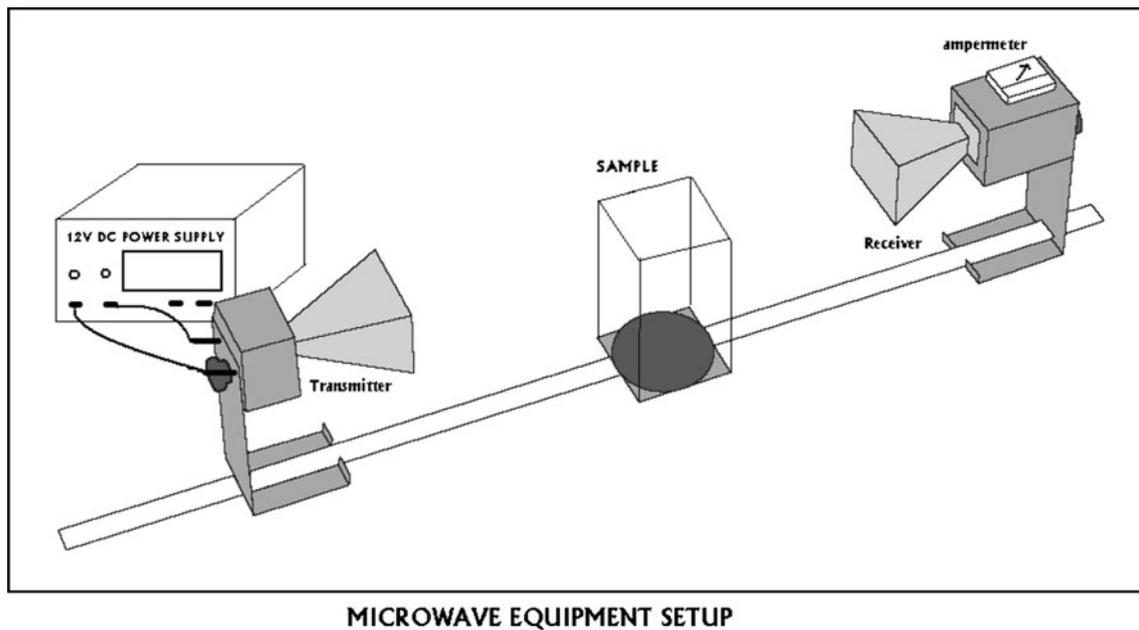
**Fig. 2** Schematic representation of the experimental system
